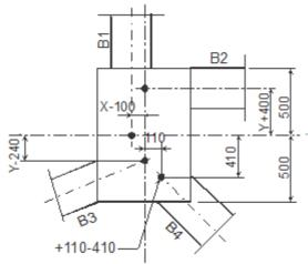
There is new field "Eccentric" in Connected Beams data.
